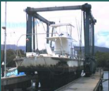
A coral viewing vessel lifted clear of the water by a travel lift. This travel lift can handle vessels up to about 30 tonnes.
