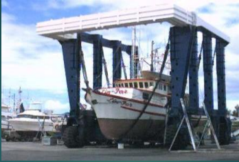
A slightly larger travel lift. This one can handle vessels up to about 150 tonnes.
