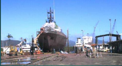
A research vessel on the slip. The rail lines supporting the cradle can be clearly seen in the foreground.
