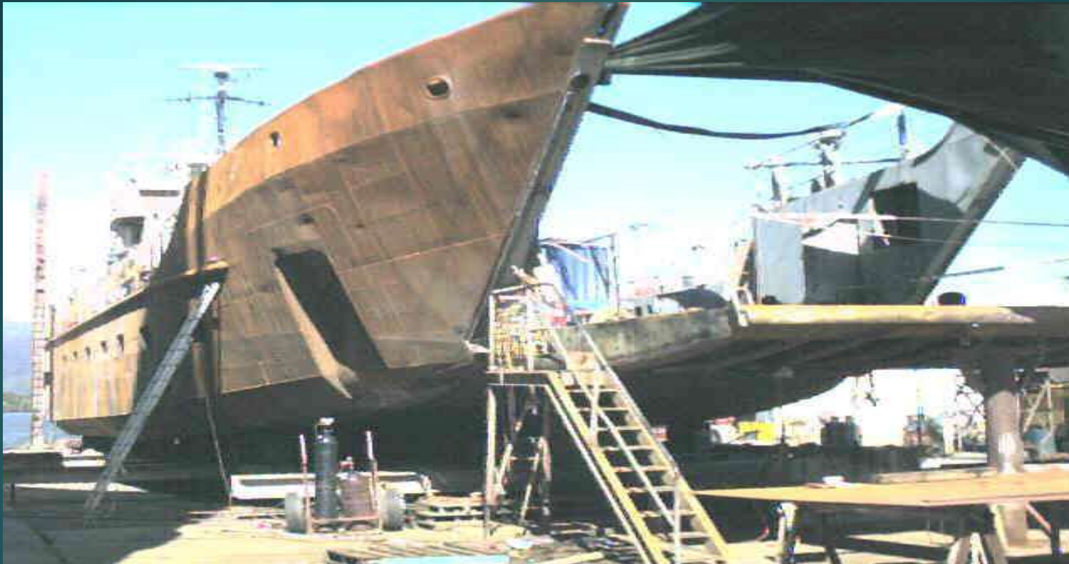
A barge on the slip. The exterior of the vessel has been sandblasted back to bare metal in preparation for painting.
